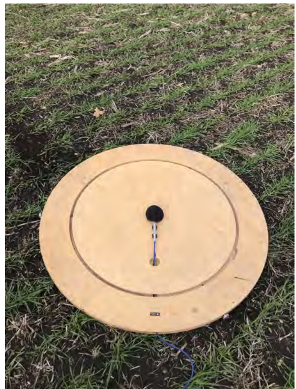
Sound Level Microphone on Board
